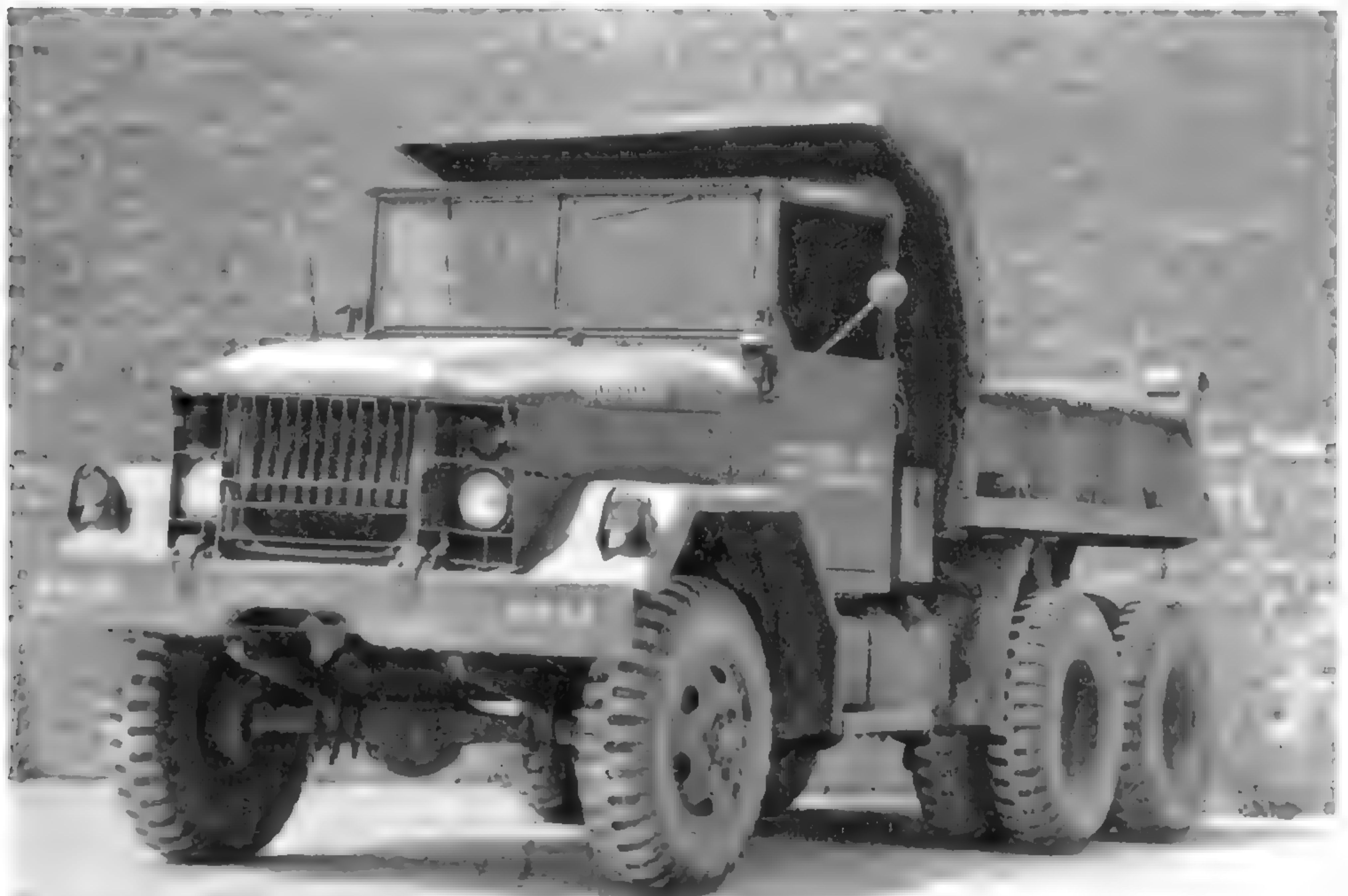
The cab protectors of the M47 and M59 were removable to reduce shipping height. The close positioning of the rear of the bed and the rear wheels caused some problems in the eyes of some of the test personnel. (Photo courtesy of the Patton Museum)
